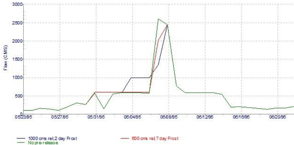
Figure 40: Outflow from Oldman Reservoir (May-June 1995)
