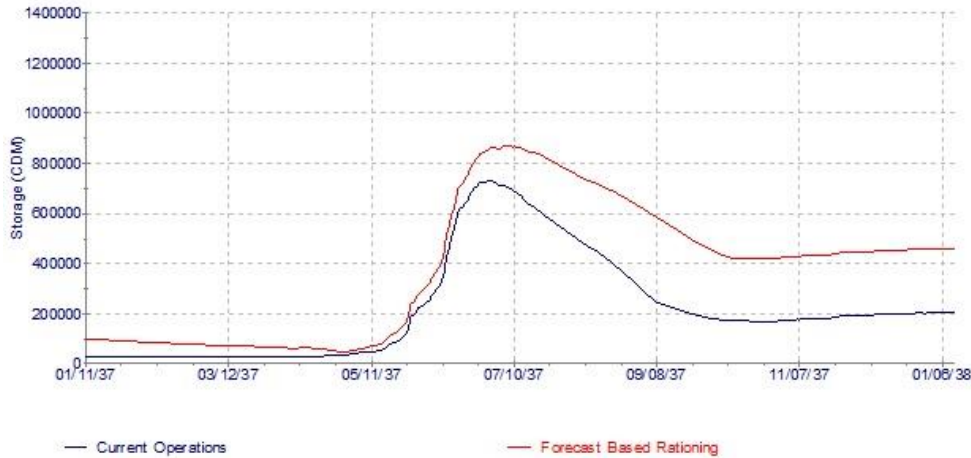
Figure 35: Storage in ESRD reservoirs after the 1936 drought (1937-1938)
